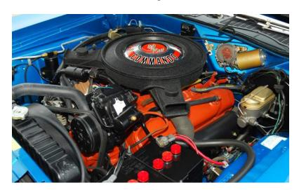
One unique aspect of this car was the single 4bbl carb, a Carter AVS model that was superceded in 1971 with the 3-2 Holley Six Pack layout on Chrysler's performance 440 engines, making the 440-4 'cuda a one-year only offering.
